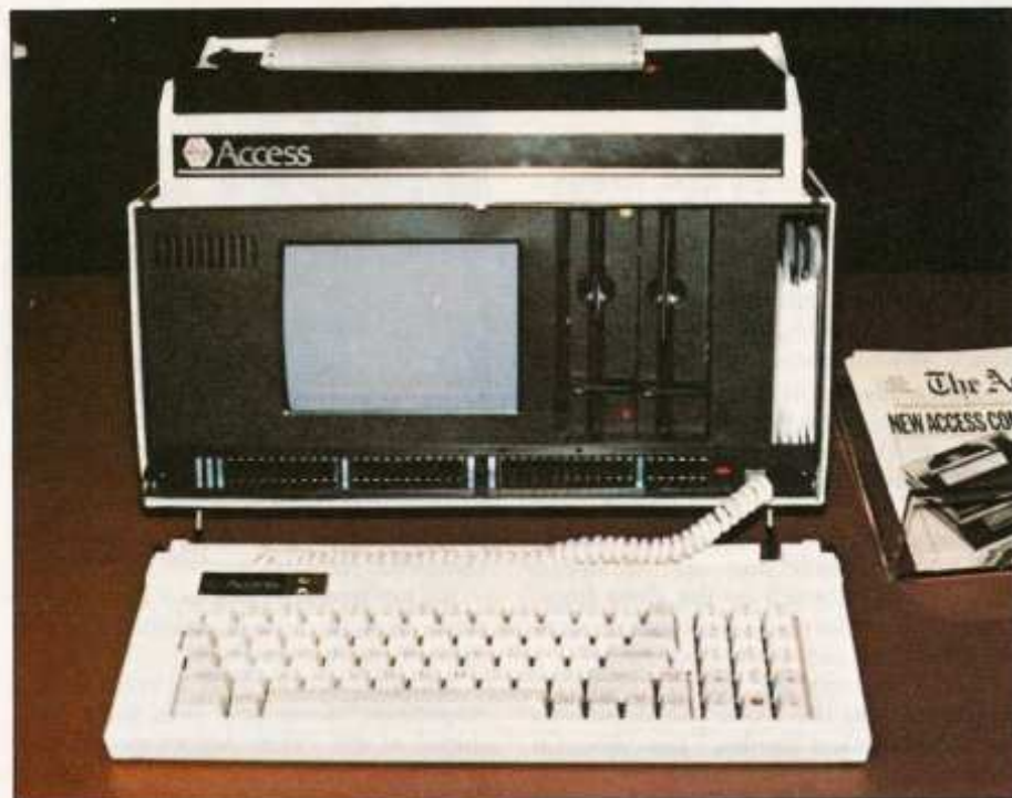
The Access computer has a detachable keyboard, 7" screen, two disk drives and built-in 80-col. printer.
