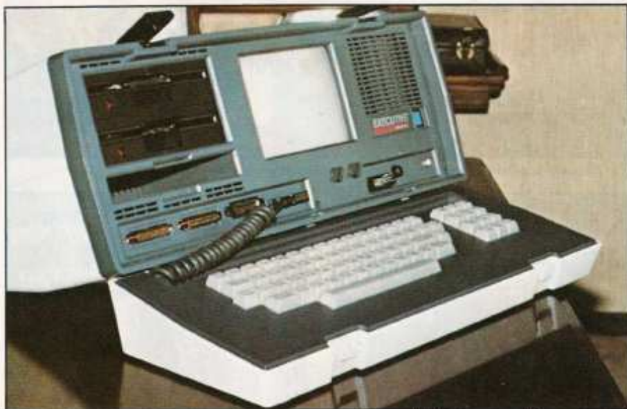
The Osborne Executive has a 7" screen, two compact disk drives, and improved housing.
