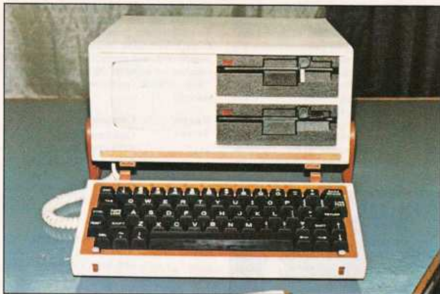
The Attache from Otrona Advanced Systems boasts bit mapped graphics, 7" screen, and a very compact design.
